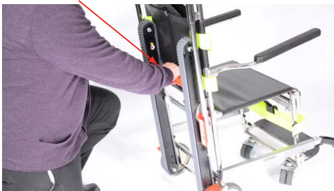
Figure 10 - Red handle for track deployment
