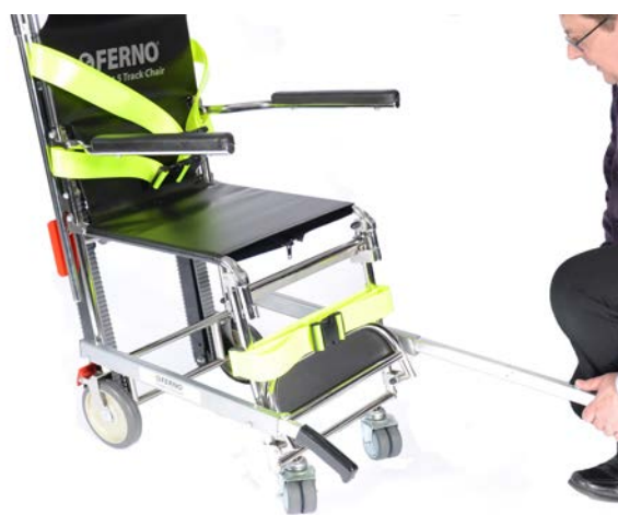
Figure 18 - Pull telescopic handle to extend
