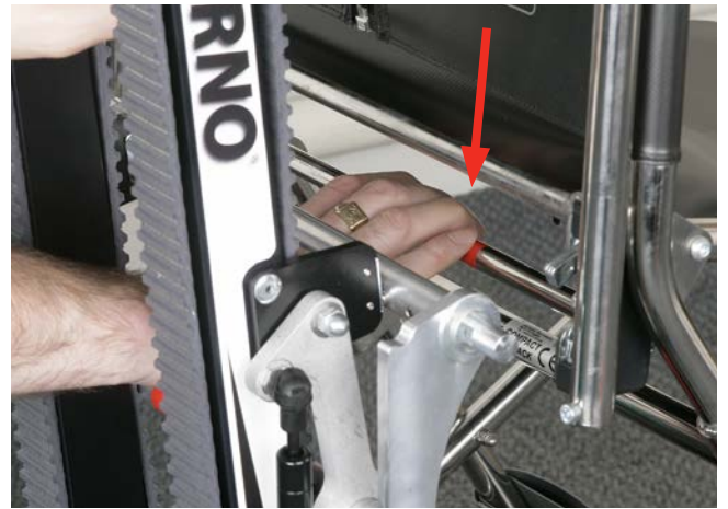
Figure 22 - Releasing Track from push-to-close latches
