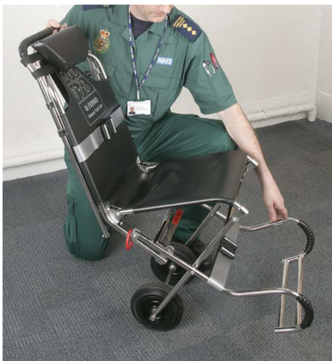
Figure 5 - Lifting up back rest whilst applying force to the foot rest
