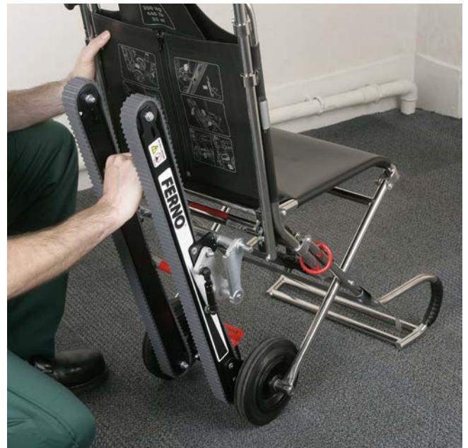
Figure 14 - Rotating Track upwards to attach to Chair
