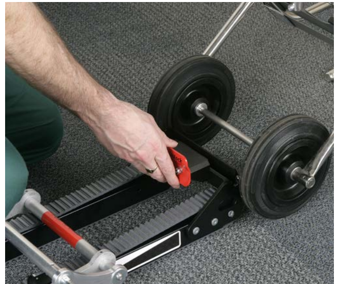
Figure 23 - Releasing the Track from the Chair
