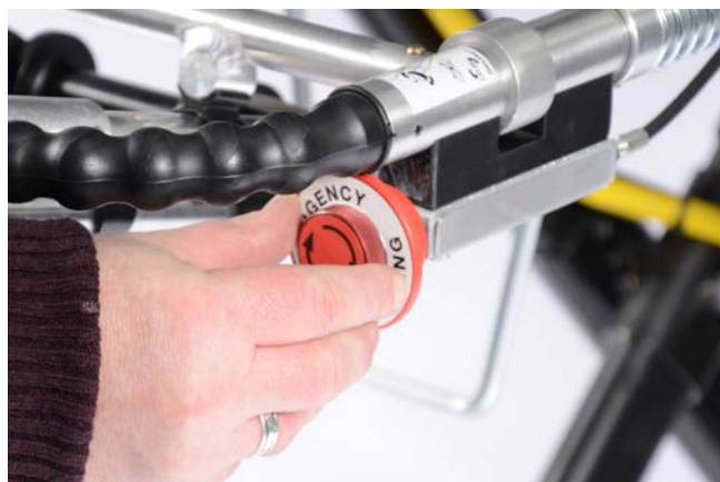
Figure 12: Turn the Manual Override knob very slowly in a controlled, clockwise direction to start lowering.
