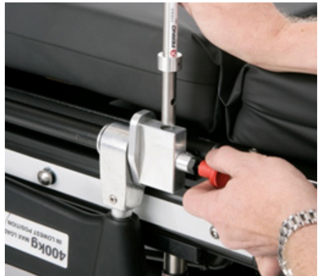
Figure 36 - Use red plunger to insert/release IV pole from block
