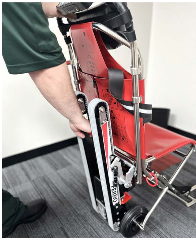
Pulling Track out for use
