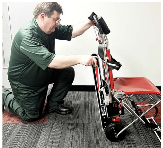
Push track towards chair to close the push-to-close latches and attach the track to the frame
