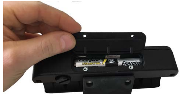
Opening the battery compartment
