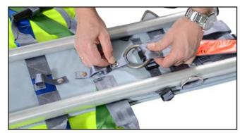
Figure 7 - Release vertical lifting rings
