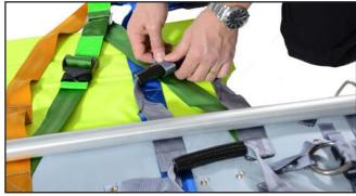
Figure 6 - Releasing Carrying Handle
