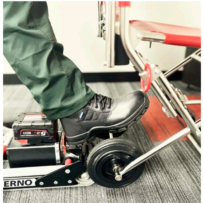
Releasing the Track from the Chair using the heel of your boot
