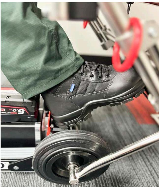
3. With the Track module laid on the ground still attached to the chair axle, straddle the track behind the chair bring your foot in under the chair and using your heel of your foot, pull back on the RED release handle on the Track module to disengage the axle locking mechanism and then lift the Chair out of the axle locking mechanism.
