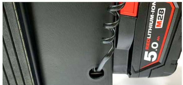
**Connecting the cable to the motor housing**
