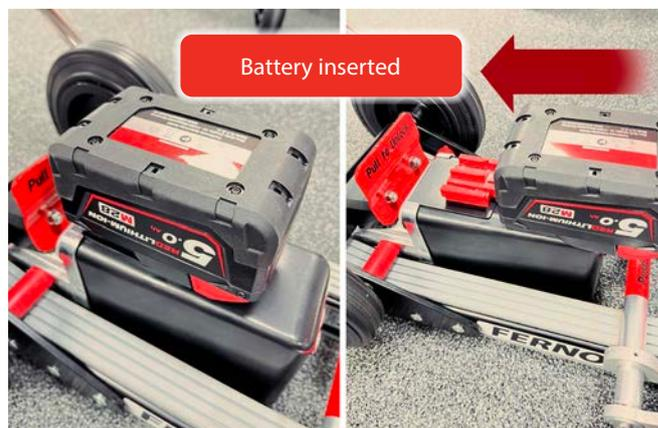
Battery attached to motor
