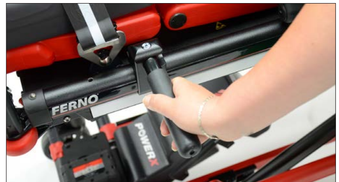
Unfold fully until clicks in place
