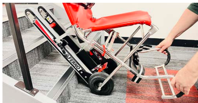
Tip the chair upwards whilst using the "+" button to bring the chair nearer to the bottom step, to then give more room to manoeuvre around the landing
