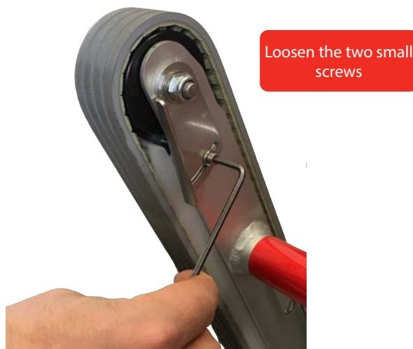
Figure 5 - Loosen the two small screws
