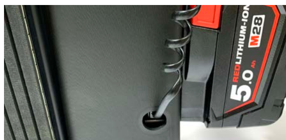
Connecting the cable to the motor housing
