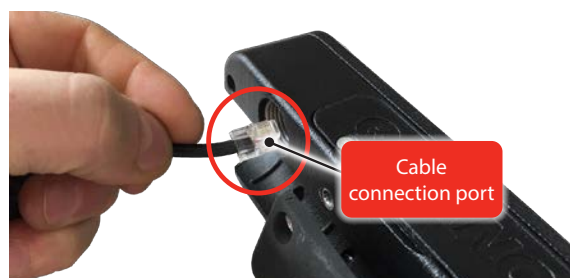
Connecting the cable to the connector port
