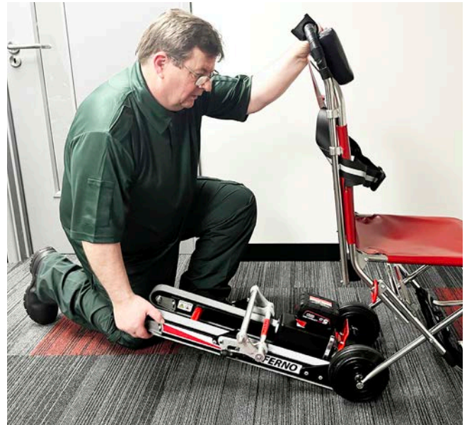
Bring the track up towards the back of the chair to lock in place
