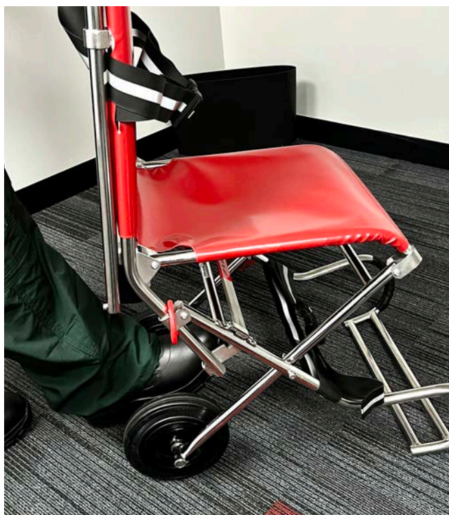
Release the locking bar to allow Chair to fold
