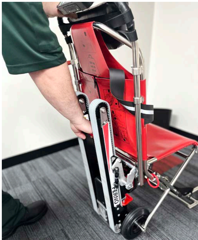
Pulling Track out for use
