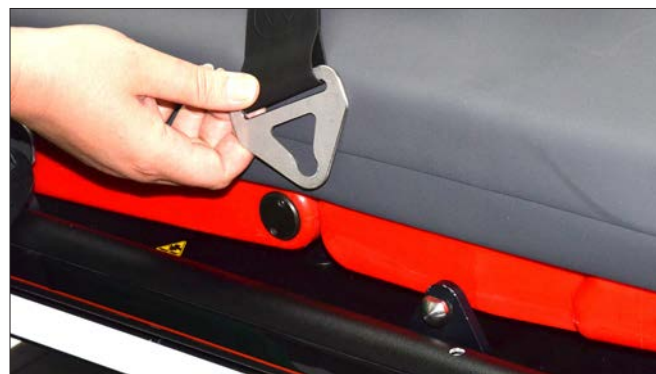
Strap tang with fixing hole
