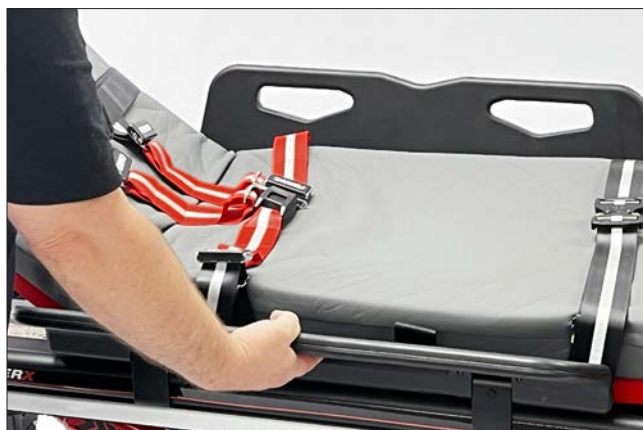
Moving SX cotside whilst depressing lever
