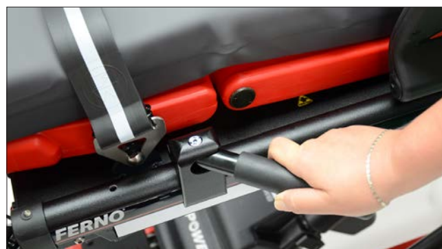
Pull towards end of trolley to unlock, then pull towards you to unfold
