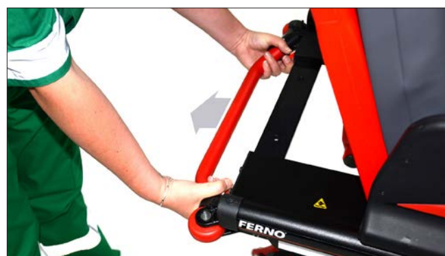
Ensure telescoping frame is locked by pulling slightly towards you after shortening
