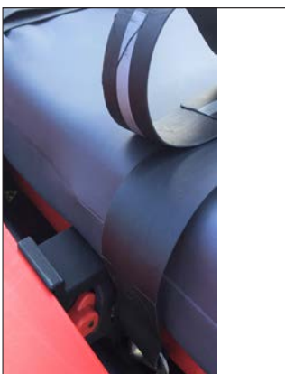
Ensure Scoop fins are under the holding plates
