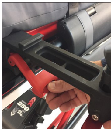
Attaching fixing bracket to siderail interface
