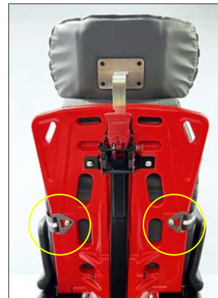
4-point harness attachment at back of backrest
