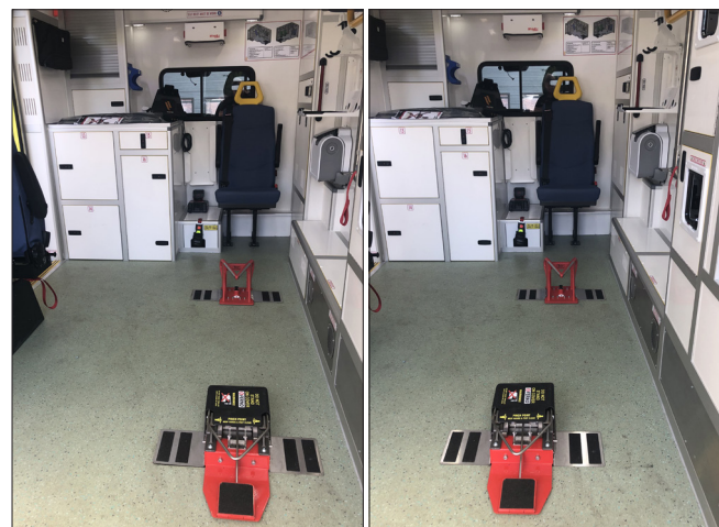
Foot-end SlideLock movement
