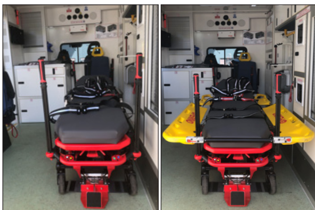
POWERX with Split Scoop attachment, SlideLock moved to B position
