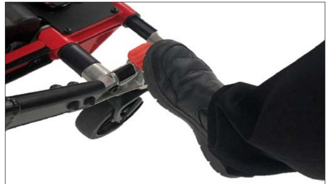
Disengaging wheel brake push forward and down
