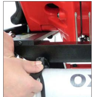
Securing straps on O2 holder
