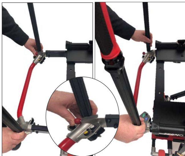
Push frame in to shorten whilst pushing in both red knobs. Once frame has fully shortened, let go of the two red push knobs and lock the frame by pulling slightly towards you
