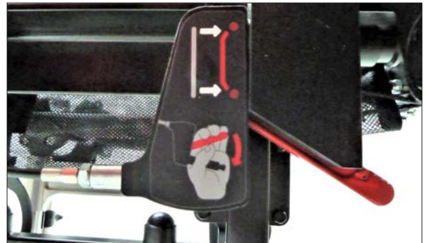
Location of manual override handle at head-end
