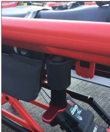
Locking arm unlocked
