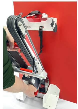
Push forward and lift up to remove Track
