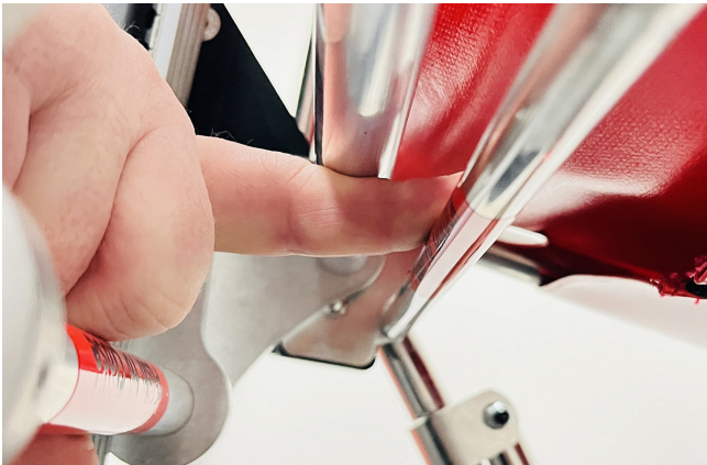
Releasing Track from push-to-close latches
