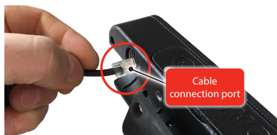
Connecting the cable to the connector port
