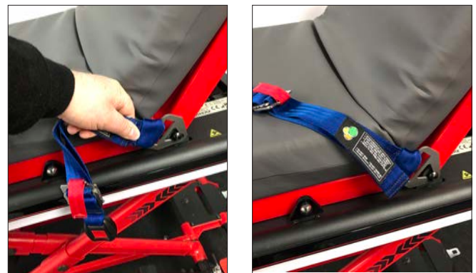
Attachment of lower ACR fixing straps to fixing stud at base of backrest either side of the trolley
