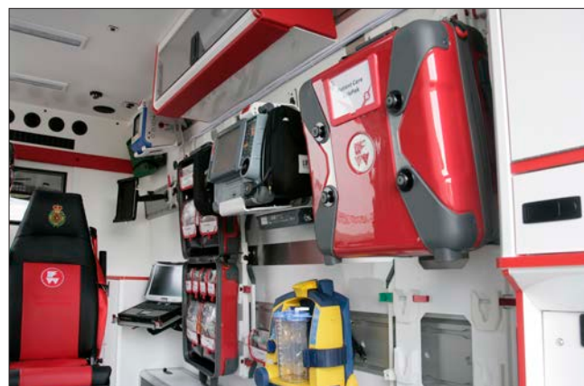
Ferno's IPTS iNTRAXX wall track bracket system
