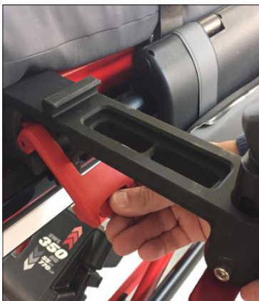
Attaching fixing bracket to siderail interface
