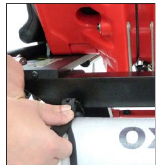
Securing straps on O2 holder
