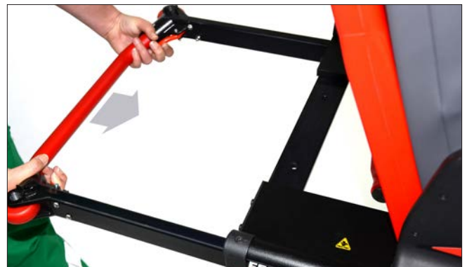
Push frame whilst squeezing both levers
