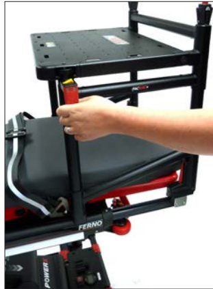
Twist the locking handle towards you
