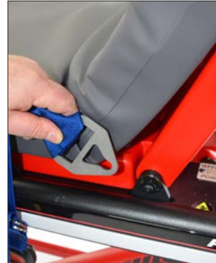
Attachment of lower ACR fixing straps to fixing stud at base of backrest either side of the trolley
