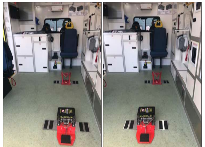
Foot-end SlideLock movement
