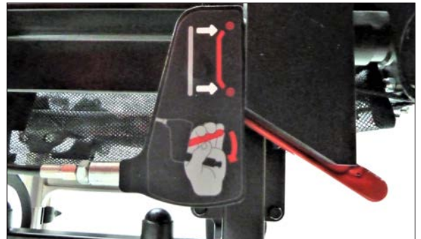
Location of manual override handle at head-end
