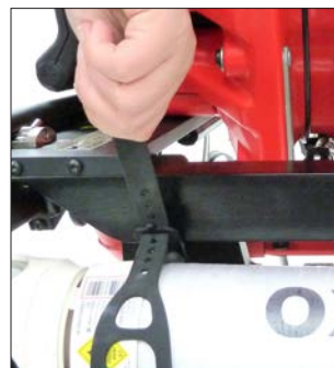
Securing straps on O2 holder
