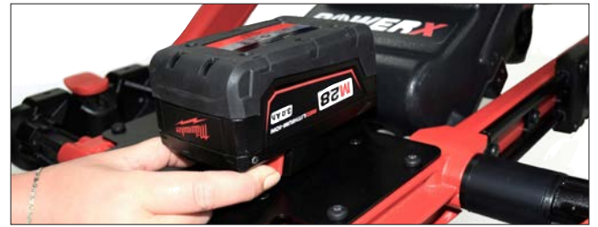
Removing battery pack
